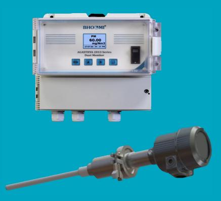
**BI 7000 Tribo Dust Monitor** is a single-point/basic functionality particulate monitor employing charge induction sensing for reliable continuous monitoring of particulate in stacks, ducts, and pipes. Applications include filter leak detection, cyclone overflow, and powder flow/no flow.
